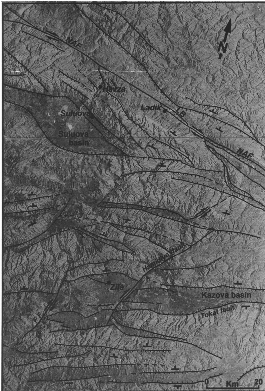
Fig. 2. Interpretation of a mosaic of SAR ERS images (negative view, ascending orbit, looking ENE) of the Havza area (location in Fig. 1c). FF, strike-slip fault; LB, Ladik Basin; NAF, North Anatolian Fault. T patterns represent dip and strike of major tilted blocks.
